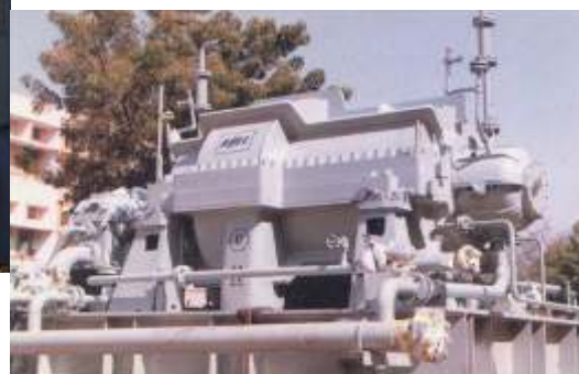
Fabricated compressor for inert gas application
