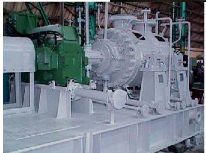
Isomerisation compressor for a refinery in Iraq
