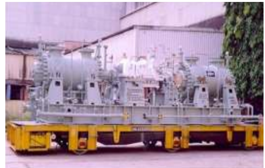
Double ended steam turbine driving LP & HP compressors for DHDT Service
