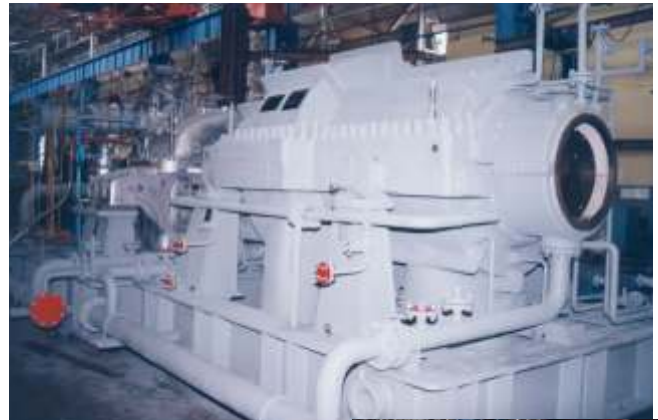
Fabricated wet gas compressor for refinery application
